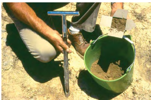
Figure 5.3. Example of a soil probe, mixing bucket, and soil box filled with soil.
