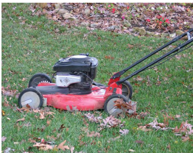
Figure 8.4. A mulching mower being used to recycle both grass clippings and tree leaves in a single mowing event.
