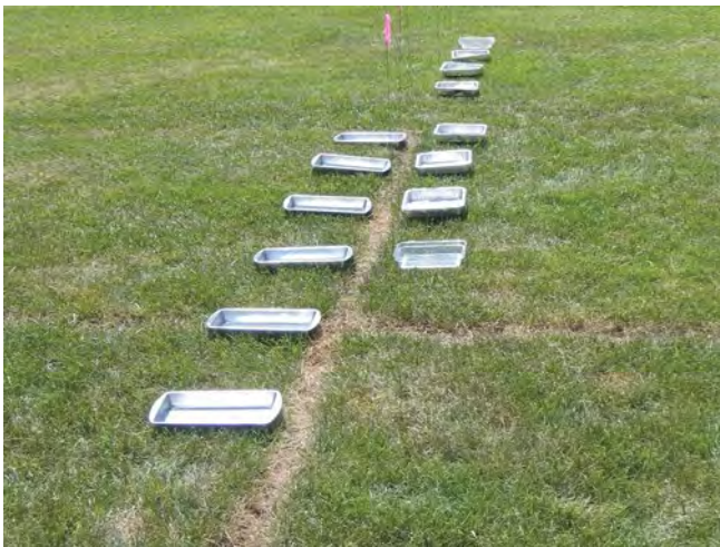
Figure 10.9. Fertilizer catch pans are being placed at regular intervals in order to determine the fertilizer's effective distribution width.
