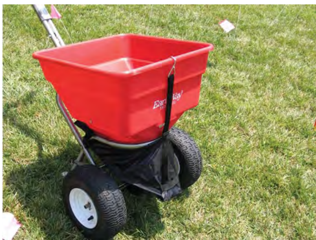
Figure 10.12. This rotary spreader is equipped with a collection bag to capture all granular product that is applied during calibration.
