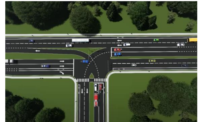
Figure 22: Example of a Continuous Green-T Intersection
